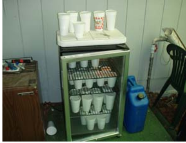
Wine refrigerator with larval rearing chambers inside and fresh stream water beside refrigerator in blue 5 gallon container.
